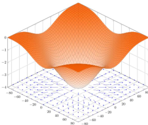
Figure 2.12: A surface and its gradient vectors
