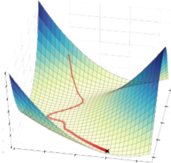
Figure 2.16: Path of several iterations of gradient descent
